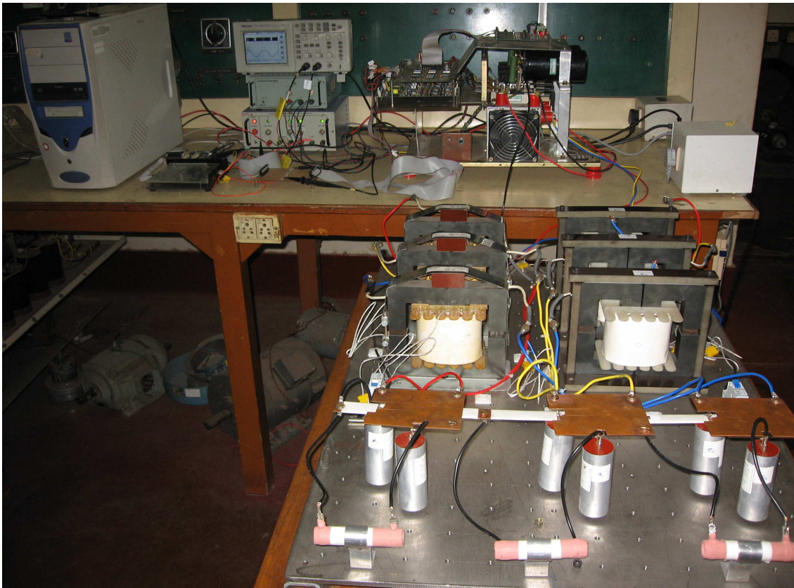
Figure C.15: Complete Physical Test Set-Up; for LCL Ferrite Core Inductor
